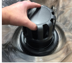
Pull Up to Remove Floater Assembly
