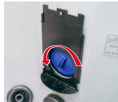
Turn Filters Counter-clockwise to Remove
